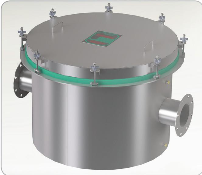
Camfil CamContain FB-R (gel seal) and GB-R (gasket seal) Housings are designed for use in critical processes where hazardous airborne materials must be prevented from escaping to the atmosphere. Air filters may be replaced from the topside of the unit using a control barrier to protect change-out personnel from contaminants within the housing or captured by the filters. The unit may be mounted vertically or horizontally.
