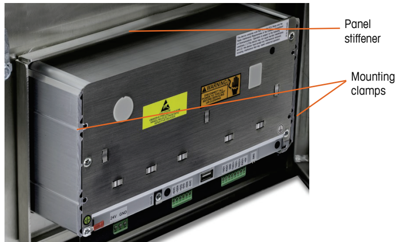
Figure 2-6: Panel Stiffener Bracket Installed
