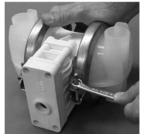
Step 8. Figure 8 Use a 11 mm (7/16") wrench to remove one set of clamp bands that secure one liquid chamber to the one-piece center section.
