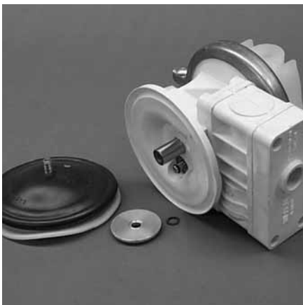
Step 11A. Figure 11A NOTE: Due to varying torque values, one of the following two situations may occur: 1) The outer piston, diaphragm and inner piston remain attached to the shaft and the entire assembly can be removed from the center section.
