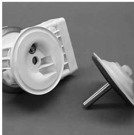
Step 11B. Figure 11B 2) The outer piston, diaphragm, inner piston, and disc spring separate from the shaft which remains connected to the opposite side diaphragm assembly. PTFE-fitted pumps come standard with back-up diaphragms (not shown). NOTE: Disc spring not shown on Figure 11B .
