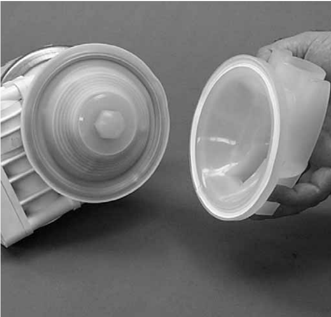
Step 9. Figure 9 Lift the liquid chamber away from the center section to expose the diaphragm and outer piston.
