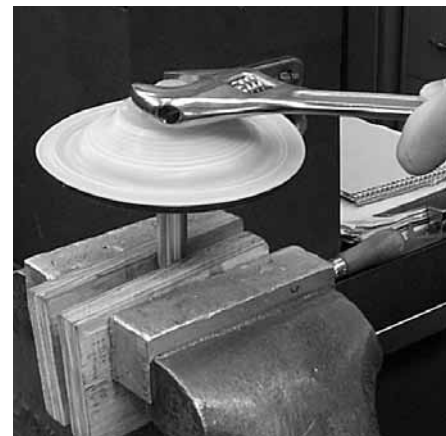
Step 12. Figure 12 To remove the diaphragm assembly from the shaft, secure shaft with soft jaws (a vise fitted with plywood or other suitable material) to ensure shaft is not nicked, scratched, or gouged. Using an adjustable wrench, remove diaphragm assembly from shaft. Inspect all parts for wear and replace with genuine Wilden parts if necessary.
